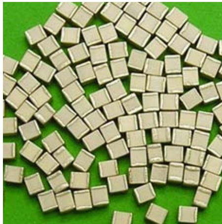
MNT12 series is high temperature RF/Microwave capacitors incorporating an ultra-stable COG (NPO) dielectric system. These capacitors are designed for continuous operating at 200°C, are low loss, high insulation resistance, and exhibit little change in capacitance over the operating temperature range. The MNT12 Series is available in voltages from 50 to 250 volts. High-reliability and burn-in testing is available as options. This Series can be supplied compliant to the EU's **RoHS** standard.
