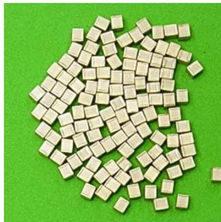
MNT11 series is high temperature RF/Microwave capacitors incorporating an ultra-stable COG (NPO) dielectric system. These capacitors are designed for continuous operating at 200°C, are low loss, high insulation resistance, and exhibit little change in capacitance over the operating temperature range. The MNT11 Series is available with 100V with a rating up to 470pF and a 50V rating up to 1000pF. This Series can be supplied compliant to the EU's **RoHS** standard.
