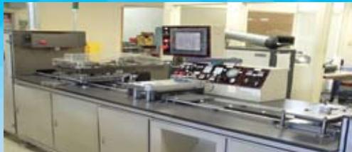
Automated Printer / Stack and Laminate
