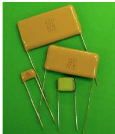
on AFM's industry proven high temperature HNT/HXT Series of capacitors. These capacitors have operating voltage ratings of 500 volts up to 4000 volts. The VNT/VXT Series is designed using a high insulation resistance, high dielectric constant barium titanate dielectric system.
